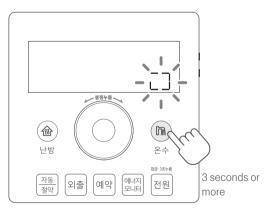
1. When power is on, press the [hot water] button to turn on the hot water system.
