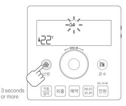
1. When power is on, press the [heating] button to turn on the heating system.
