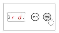
1. Press and hold the [Select] button for at least 3 seconds while the power is off (---), and (- d) is shown on the display.
