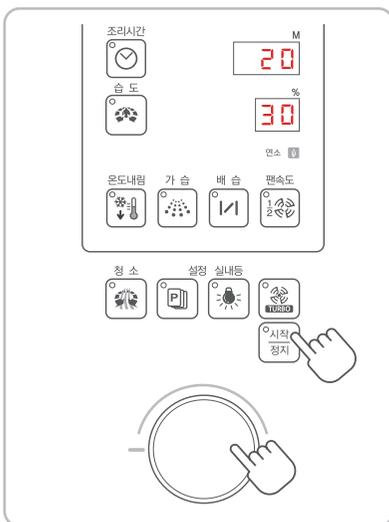
4. Turn the adjustment handle to set the time, then press the [Start/Stop] button to finish cooking.
