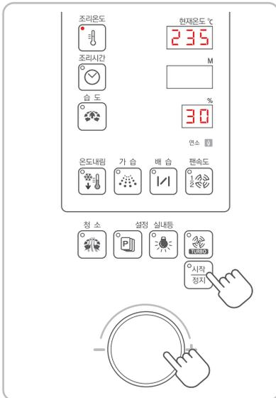
2. Turn the adjustment handle to set temperature and humidity, then press the [Start/Stop] button.
